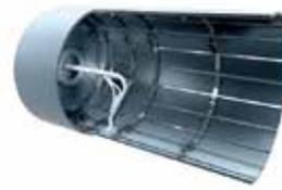
Destroy the condensate film created on the inner surface thus enabling higher heat transfer through convection between steam and the inner cylinder surface
