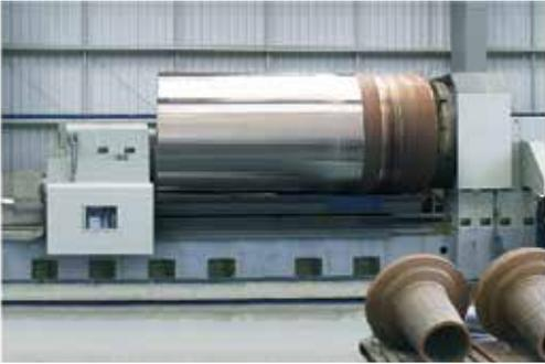
CNC Horizontal Lathe
