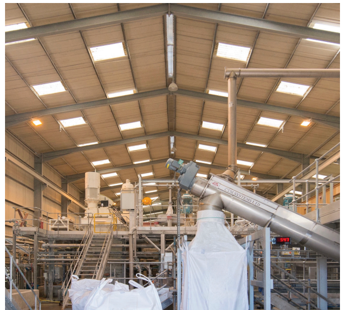
Figure 1: FiberLean MFC onsite scalable modules center around robust grinding technology. High-throughput continuous operation—Low maintenance costs and high uptime (>95% plant availability)—Chemical-free process—Highly-automated modular plant design with online monitoring.
