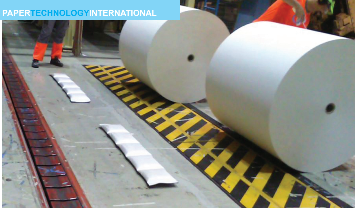
Figure 3: Braking Pad on winder deck.
