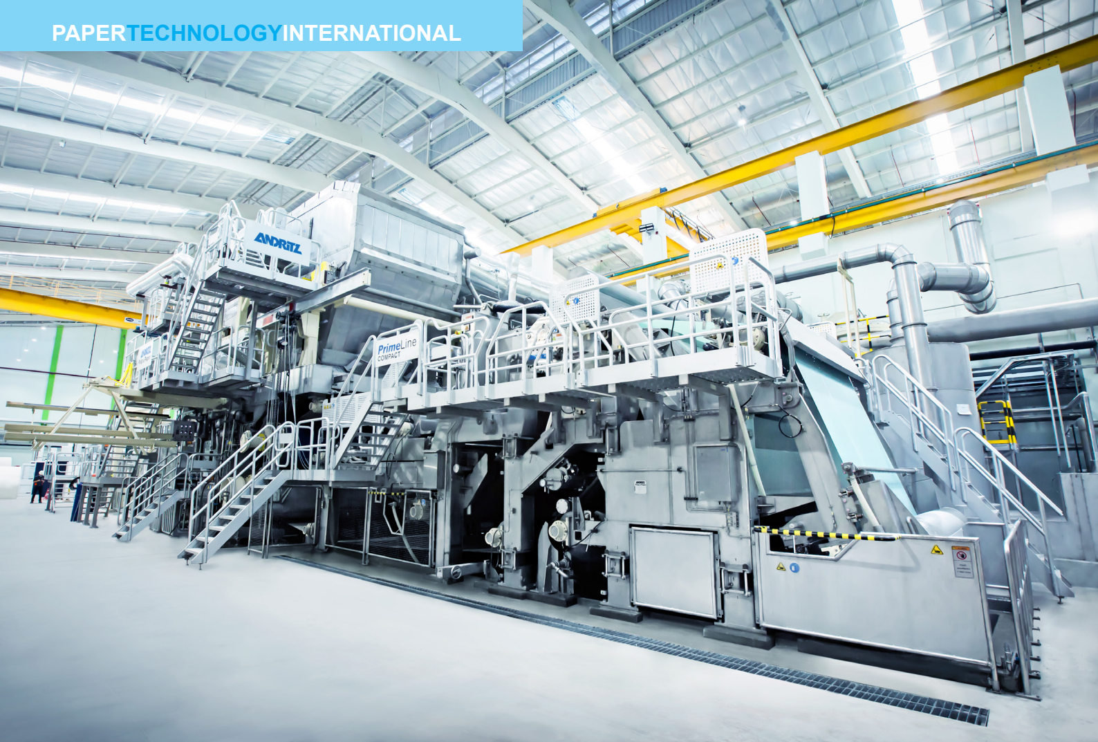
Figure 5: PrimeLineCOMPACT tissue machine with resource saving components.
