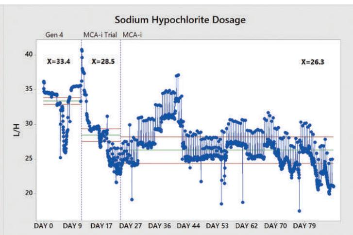
**Figure 5: Phase 2 Trial Conversion Evaluation of MCAP and Sodium Hypochlorite Dosage Rates.** Both chemical dosage rates were reduced further while the MCA headbox residuals noted in the trial phase were maintained (Figure 4).
