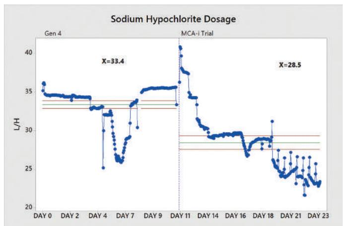
**Figure 2: Phase 1 Trial Evaluation of MCAP and Sodium Hypochlorite Dosing Rates. For the MCA-i trial, both chemical flow rates were reduced while maintaining a slightly higher headbox MCA residual (Figure 1) as compared with the Gen 4.**
