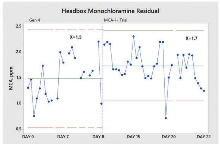
**Figure 1: Phase 1 Trial Evaluation of Headbox MCA Residual. When comparing the performance of MCA-i with the Gen 4, slightly higher MCA residuals (13.3%) were achieved.**
