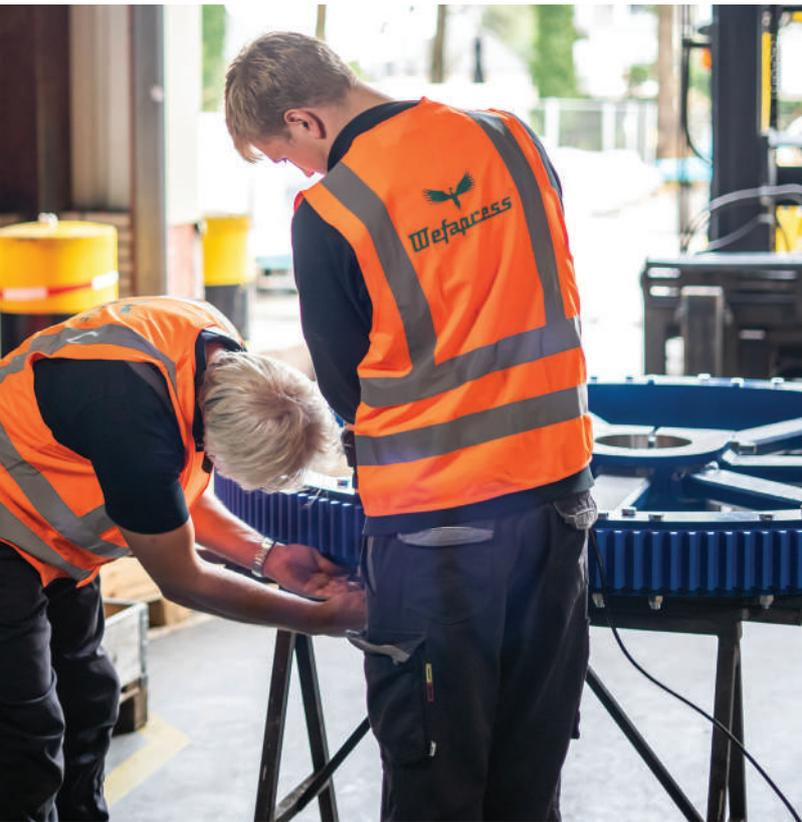
**Figure 5: Gear wheel mounting service at paper mill.**
