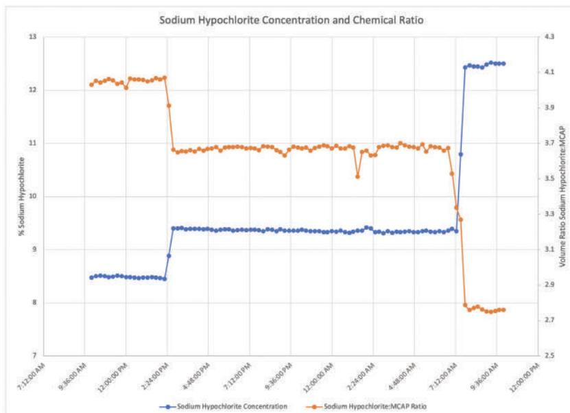
**Figure 6: Phase 2 Trial Conversion Evaluation of Hypochlorite Sensor.** The sodium hypochlorite activity over a 24-hour period is shown. As a new delivery was transferred to the run tank, the concentration increased from 8.5% to 12.5% and the MCA-i unit automatically adjusted the MCAP : sodium hypochlorite ratio to maintain a stable MCA solution.
