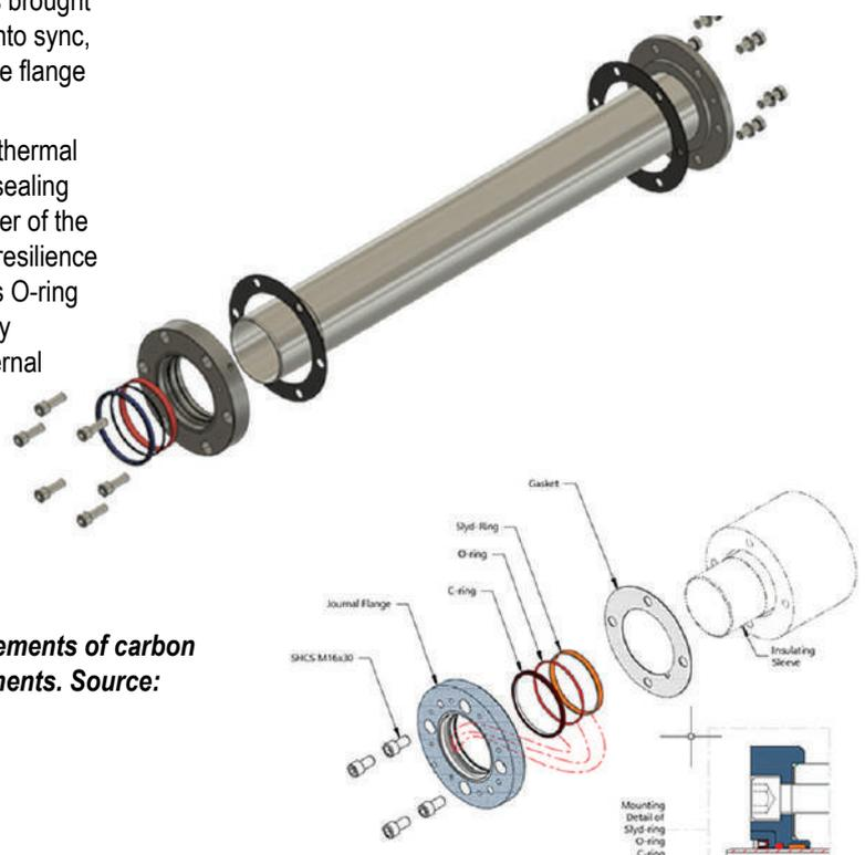
**Figure 3: This innovative insulating sleeve employs elements of carbon steel and stainless steel, along with static sealing elements. Source: Deublin Co.**
