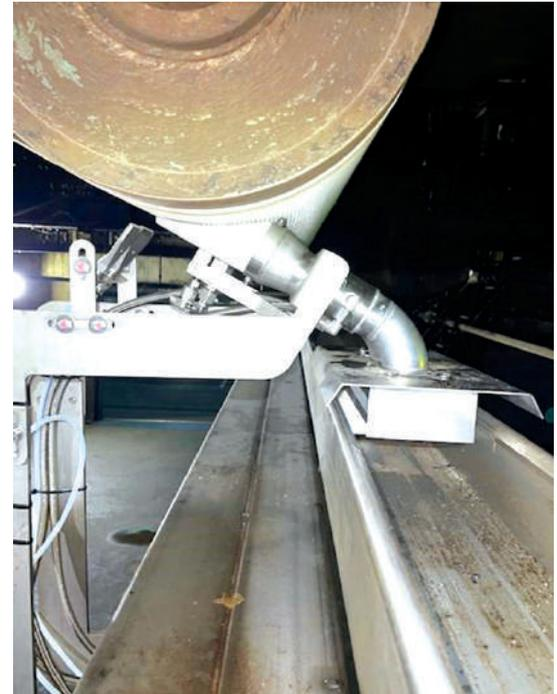
**Figure 2: Power Cleaner 2.0 on Bottom Fabric.**
