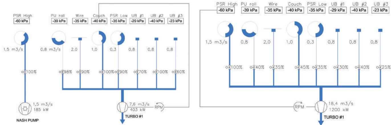
Figure 2a & 2b: Combining all vacuum consumers with different vacuum levels to one unit can destroy system efficiency due to expansion/throttling losses.
