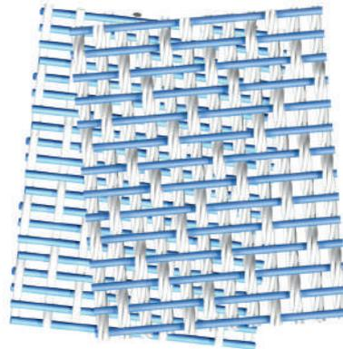
Figure 2: Combination twisted / mono.
