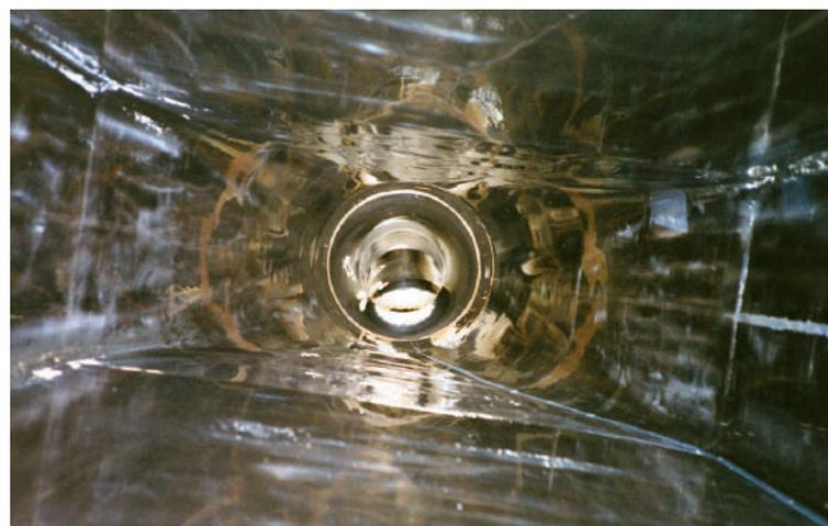
**Figure 7: Same headbox after successful cleaning, barium sulphate scale removed.**
