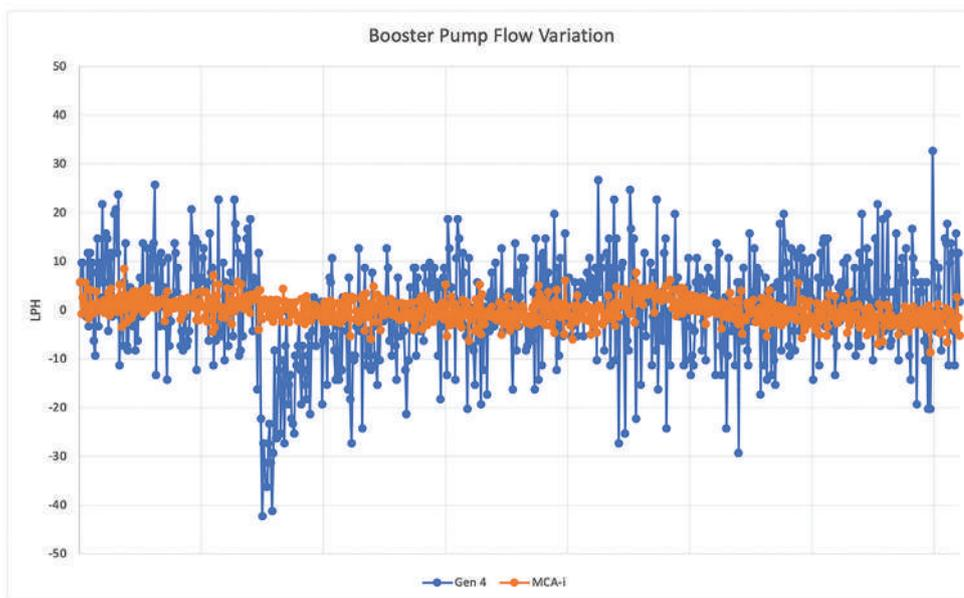
**Figure 6: Phase 2 Trial Conversion Evaluation of the PID Flow Control Valves.** The water booster pump variation over a 12-hour period was compared between the Gen 4 unit and MCA-i. The flow variation was reduced by 75% due to the use of the PID flow control valves in MCA-i.
