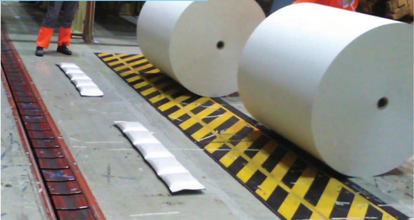
Figure 3: Braking Pad on winder deck.
