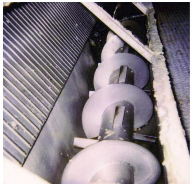
**Figure 5: The same conveyor screw treated with pitch control agent.**
