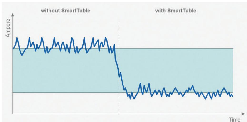
Figure 7: example for couch roll amps reduction.
